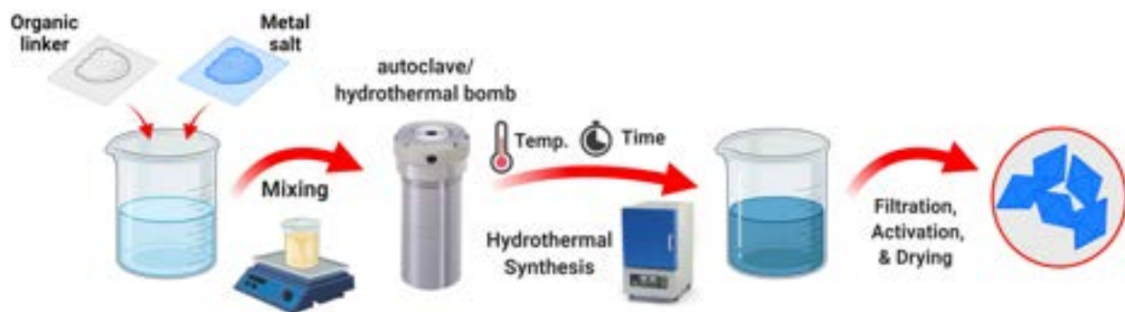
Figure 2.8 Conventional hydrothermal/solvothermal method for MOF synthesis.
