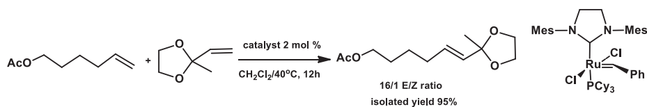
Fig. 21.125: Cross-metathesis of the methylvinylketone ketal with 6-acetyl-1-hexene.
